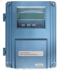
transducers on the pipe, enter the pipe and medium parameter and adjust the distance between the transducers as indicated by the meter. No zeroing procedure is necessary since all transducer pairs are factory calibrated and the calibration data is permanently stored in the transducers themselves. The user interface is always automatically adapted to the actually connected transducers.
